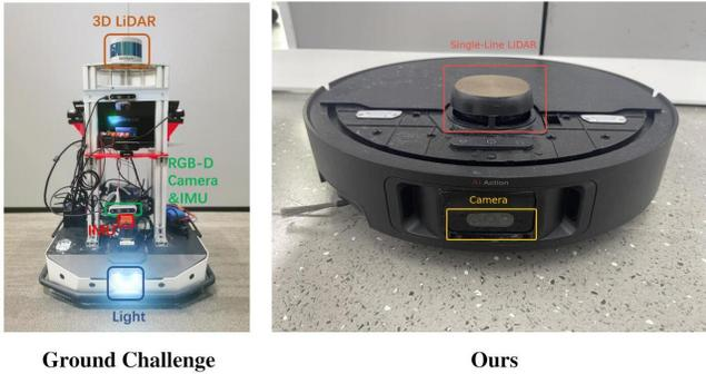
Fig. 9. Comparison of equipment used in the Ground Challenge dataset [29] versus that used in our sweeping robot system.
